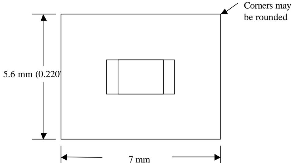
Circular holes can be used, but they would require a larger total cutout area, a diameter of 7 mm (0.275") to be certain. However, a 6.35 mm (0.250") diameter cutout is common for this size of LED, if your die-cutting and laminating processes are well registered. However, if your processes are not under control this may result in additional problems.
